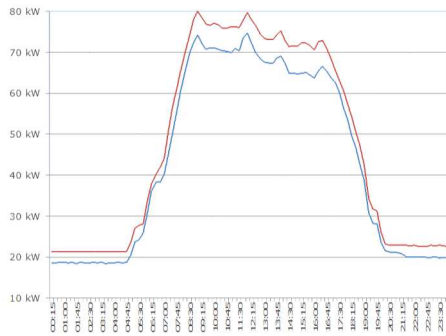
Example of power consumption in kW before (red) and after (blue) installation of the VoltControl Stabilizer.
